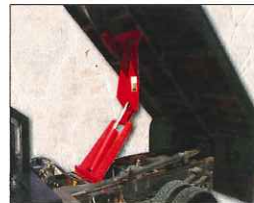
Single Cylinder for 1 ton trucks 5 to 20 ton hoist for beds from 8ft.—20ft. Long.
